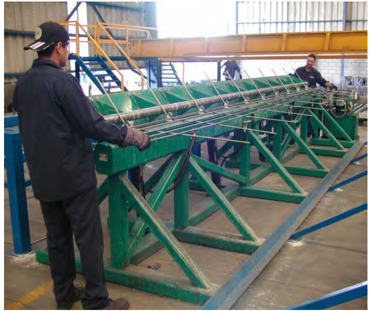
Figure 3-5: Hydraulic or pneumatic machines are used to fabricate WWR bent mats
