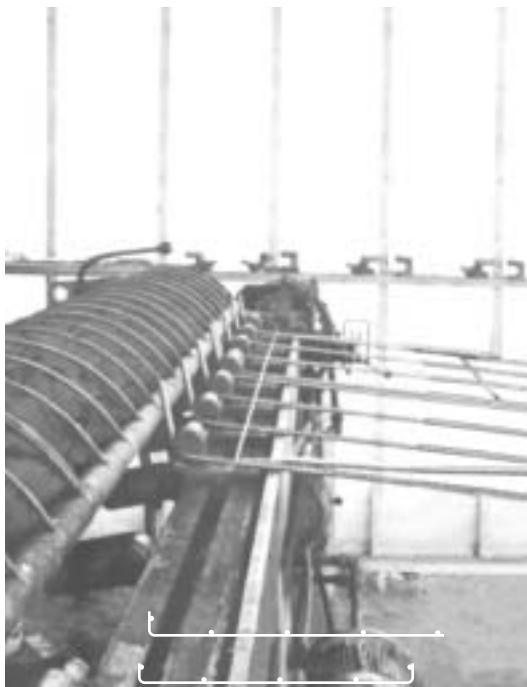
1ST & 2ND BENDS: Bending arm (left) is rotating and putting 90° bend into end of sheet. Other end of sheet next will be shaped identically.
