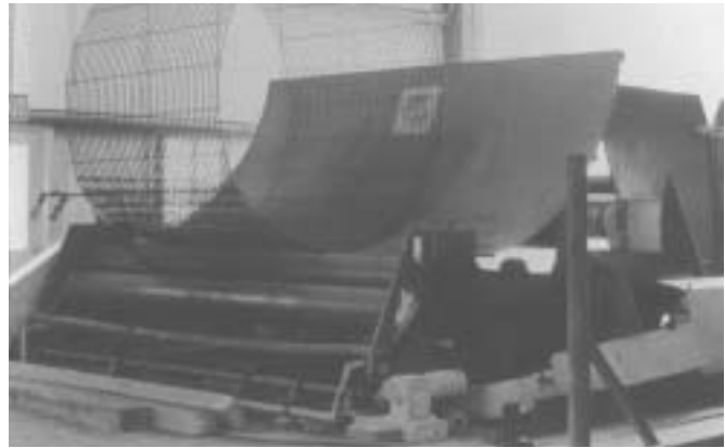
Welded Wire Reinforcement manufactured for concrete pipe.
