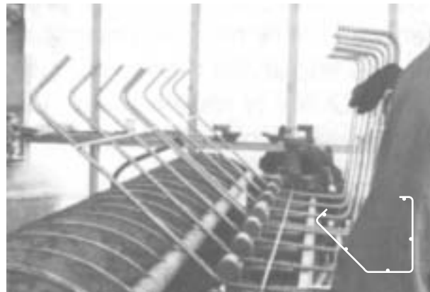
4TH BEND: Bending arm is rotating and putting the final 90° bend into fabric shape.
