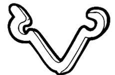
A variety of wire and plastic supports are available – many are made especially for welded wire reinforcement. Adequate spacing of supports depends on the style and size of wires. Spacings of supports varies from 2–6 feet and more depending on wire sizes and spacings.
