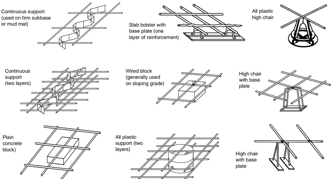
For welded wire reinforcing sheets, spacings of the individual wires should be a consideration to avoid permanent displacement due to workers walking on the reinforcement. This spacing should be 12 inches or more (up to 18 inches may be specified). If the design requirements do not allow larger spacings, then the wire stiffness and the support strength and spacings must be adequate to carry all anticipated construction loads.
