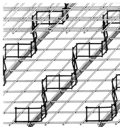
Welded wire reinforcement placed on welded wire supports.
