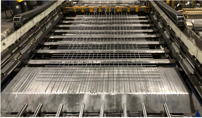
Figure 30: Output side of the WWR production line, showing a WWR mat intended for structural slab usage.
