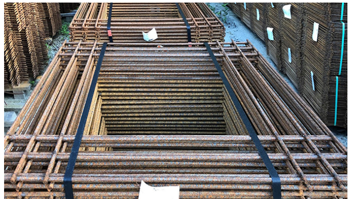
Figure 14: WWR mat bundle showing a configuration intended for the top slab of a square concrete riser structure
