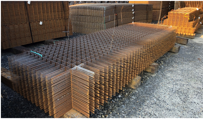
Figure 17: WWR mat bundle showing a configuration to be used in a structural slab. Notice the extended overhangs to facilitate the lap splice continuity of adjacent mats once placed in the field.
