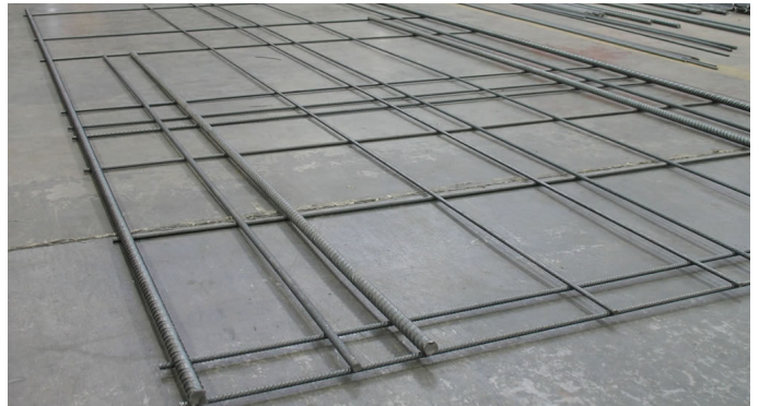
Figure 8: WWR mat with variable linewire and crosswire spacing, size, and length
