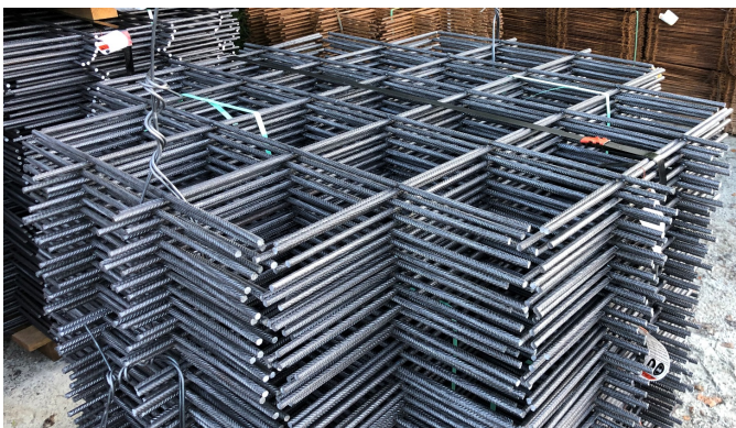
Figure 15: WWR mat bundle showing a configuration for use in a precast concrete element.
