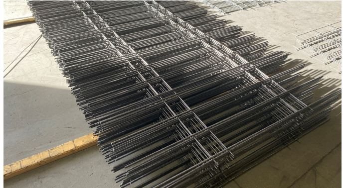
Figure 10: WWR mat bundle showing project-specific wire arrangement and overhangs
