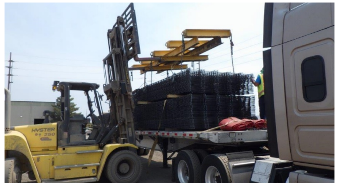
Figure 47: Forklift loading of WWR bundles onto truck
