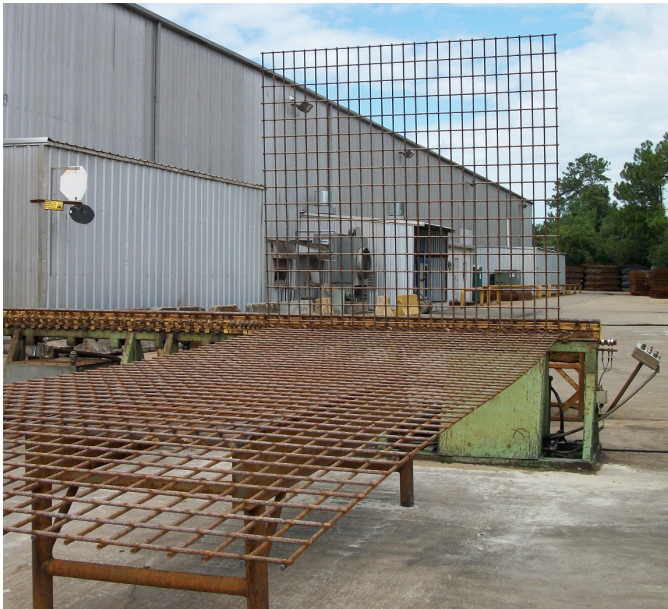
Figure 34: Bending of a WWR mat with large diameter wires
