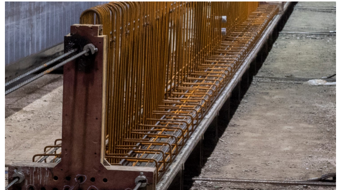
Figure 37: A precast beam stressing line populated with bent stem and flange WWR mats.
