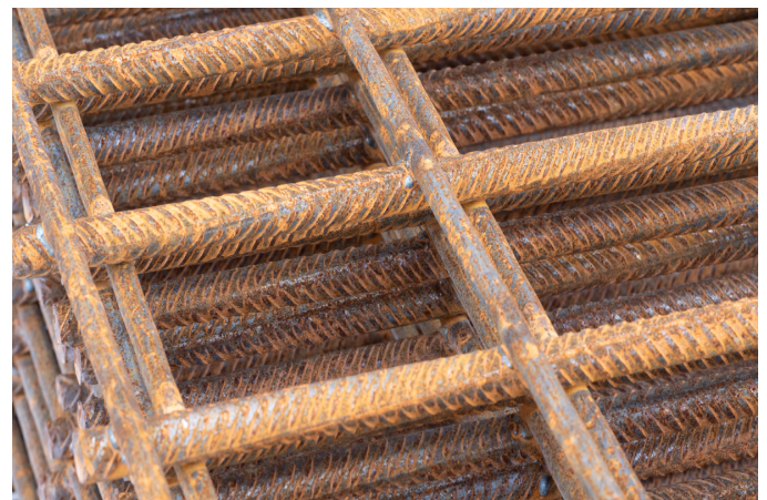
Figure 5: WWR mats in a bundle, showing deformed wires welded to plain wires. Notice the contrast in surface profile.
