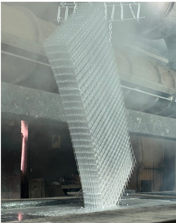
Figure 46B: Hot drip galvanizing of a WWR bundle.
