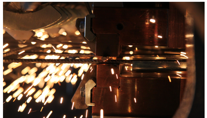
Figure 29: A close-up transverse view of wire intersections being fused by the electric resistance welding process on a modern automatic welding machine.
