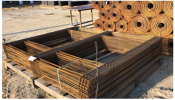
Figure 18: WWR mat bundle showing a configuration characterized by wide wire spacing.
