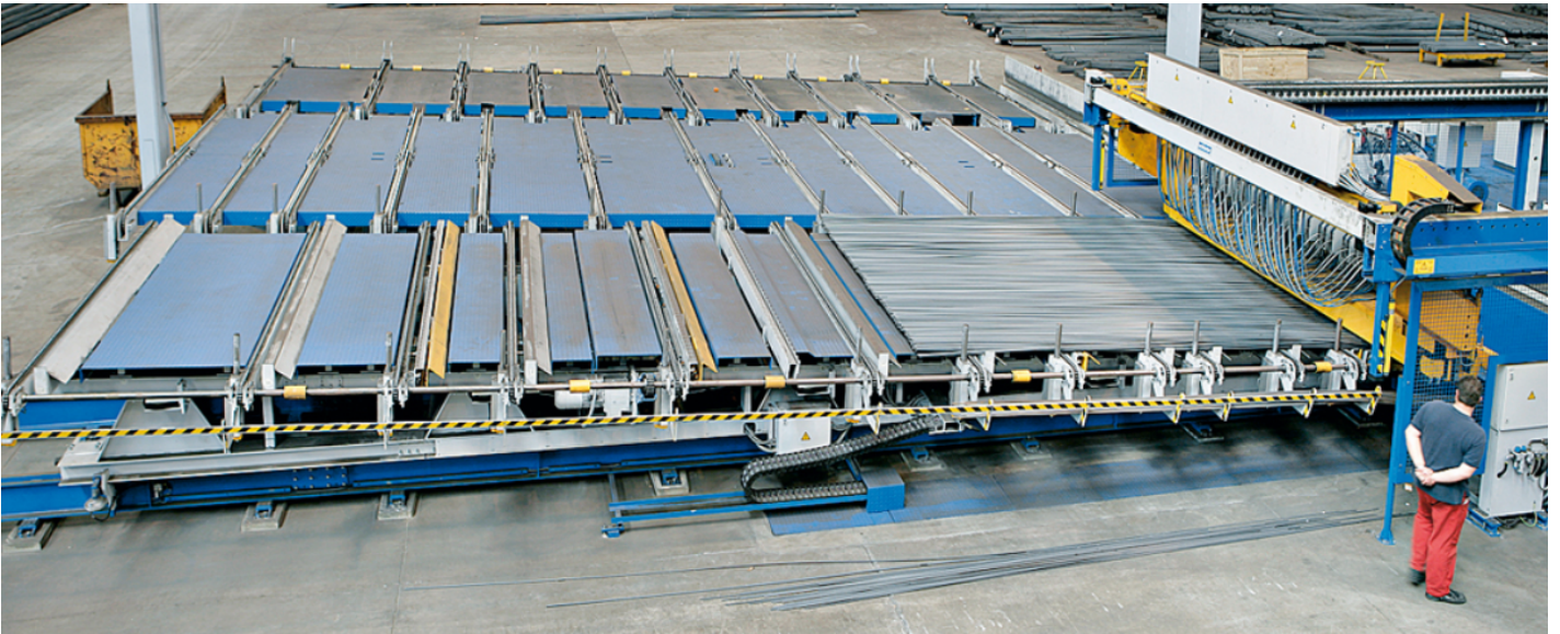
Figure 25: A view showing staging area populated with straightened and cut-to-length individual wires that will be automatically positioned and pulled through the machine. These wires will ultimately serve as the linewires on the automatically-welded WWR structural mat.
