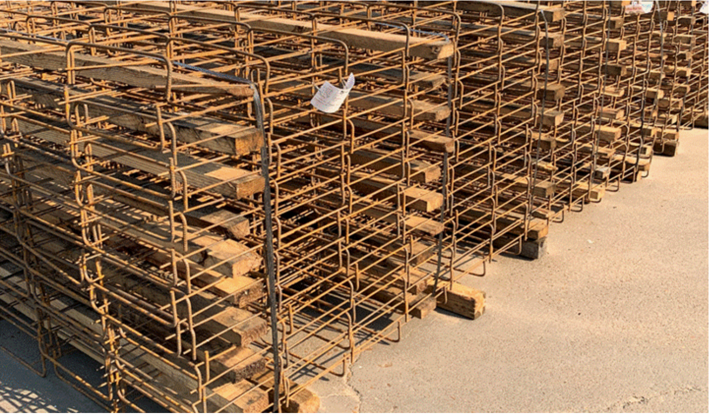
Figure 1.4: Bundles of bent WWR staged on the manufacturer’s yard in preparation for loading and shipment
