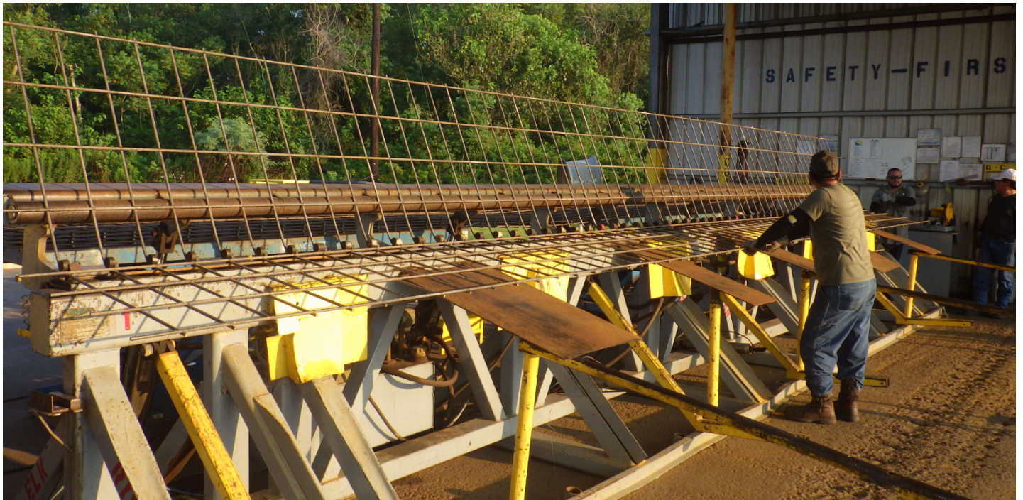
Figure 2.3: Bending Operation Step 2 – With the WWR positioned firmly, the operator enters the required bend angle at the control end of the machine, and the hydraulically-driven continuous rail contacts the WWR mat, creating a pushover effect. Because the WWR is secured so as not to be dislodged from the mandrels, cold bending of the wires results as the continuous rail starts to rotate through the programmed bend angle.
