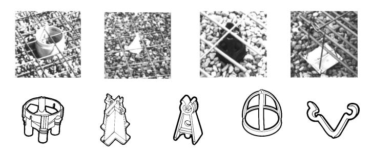
A variety of wire and plastic supports are available – many are made especially for welded wire reinforcement. Adequate spacing of supports depends on the style and size of wires. Spacings of supports varies from 2–6 feet and more depending on wire sizes and spacings.
