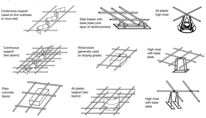
For welded wire reinforcing sheets, spacings of the individual wires should be a consideration to avoid permanent displacement due to workers walking on the reinforcement. This spacing should be 12 inches or more (up to 18 inches may be specified). If the design requirements do not allow larger spacings, then the wire stiffness and the support strength and spacings must be adequate to carry all anticipated construction loads.
