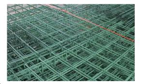
an ASTM standard for stainless steel wire and WWR. It is ASTM A1022-02. Wide
