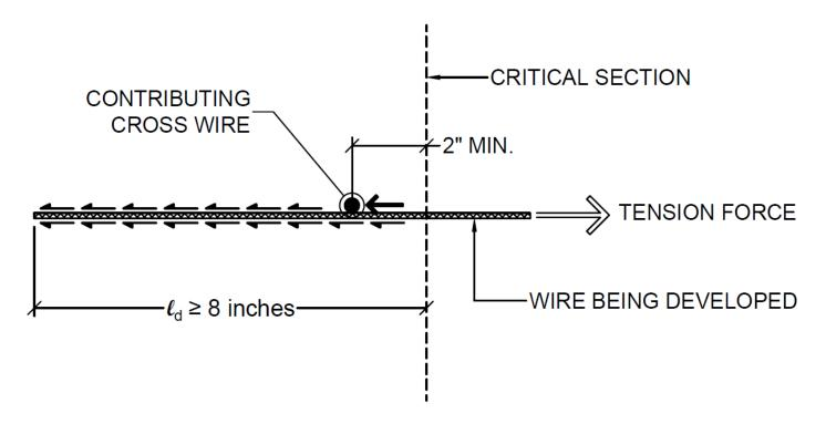
5. Upon calculation of the modified development length, and with contributing cross wires appropriately positioned within the splice region, calculate the tension lap splice length per AASHTO Article 5.10.8.5.1, illustratively represented in the diagram below as the larger of 1.3 x  $l_{\rm d}$  and 8 inches.
