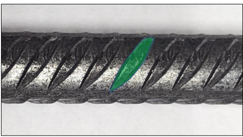
Protrusions ("ribs") are known as "positive deformation".
