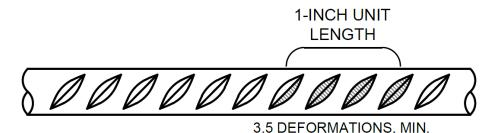
In practice, the verification of deformations per inch is on a minimum 10-inch specimen length. 1-inch equivalent lengths are illustrated here for visual reference.
