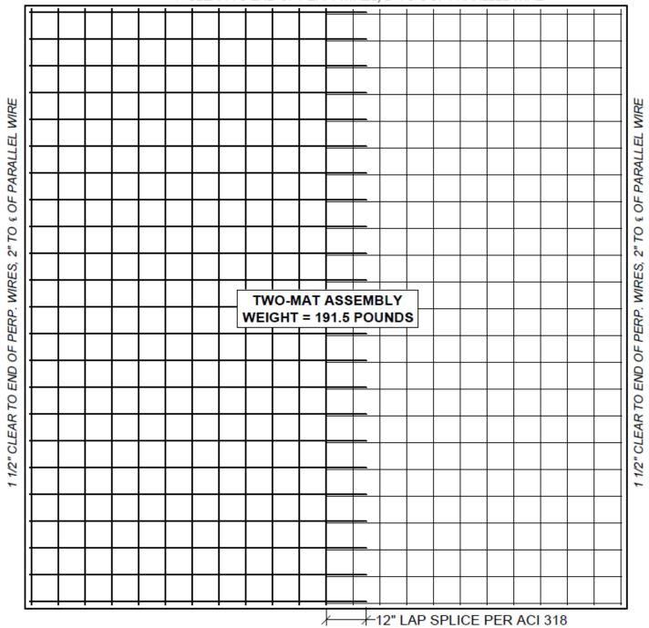
1" CLEAR TO END OF PERP. WIRES, 2" TO € OF PARALLEL WIRE
