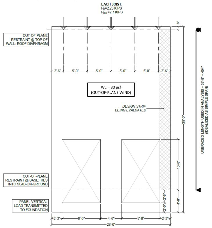
The image above shows a typical reinforced concrete tilt-up wall panel configured with two loading dock doors and supporting long-span roof framing. The wall is to be analyzed
