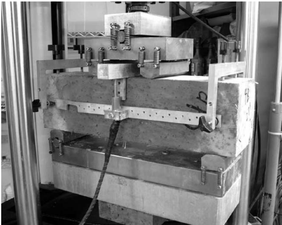
ASTM C1609 test configuration (image from ASTM C1609, ASTM International)
